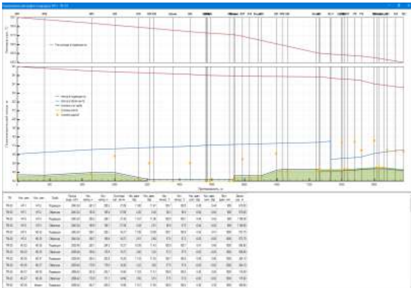
Figure 2.3. Temperature distribution in the supply and return main pipelines of the heating network
